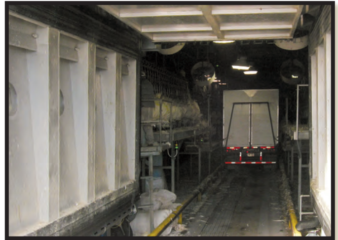
Cooper Farms three panel (CAS) system allows the atmosphere to be controlled on the truck by section. This industry-leading, cutting edge technology is the ultimate in humane stunning.
